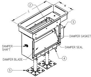
☐ FTS - FLOOR TILE SUPPORTED WITH VC PLENUM STYLE (FOR LBG 1000 STYLE BORDER)
